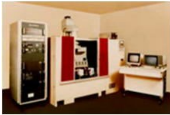
Fig-1 10:1 stepper (NIKON NSR-1010G) (Courtesy of Nikon Corporation)
