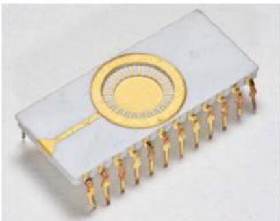
28-pin DILC (2-die package, after die attach and before cap seal)
